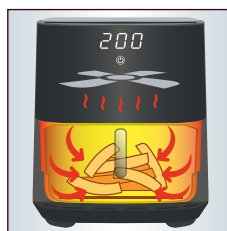
360° Air-Flow: Oil and fat free frying by hot air circulation
