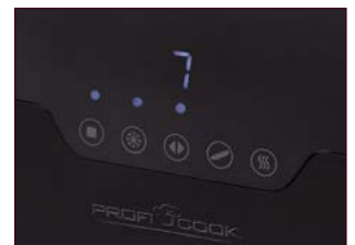
LED display (blue illuminated) with sensor touch operation
